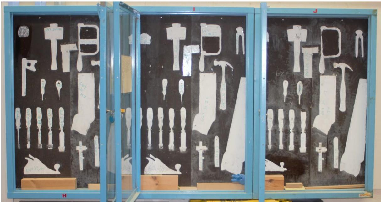
Image 1: Photograph of a Shadow Board, note the removed item can easily be identified as to where it should be replaced due to the 'shadow' left behind when the item is in use. This ensures a quick visual check would immediately identify if anything was missing during cursory and formal checks.
